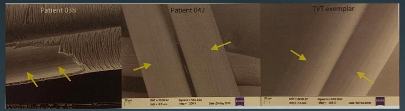
Exponent showed that this "cracking" effect was caused by tissue adherence, and it could be cleaned to expose an unoxidized, nondegraded surface
